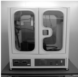
Fig. 10. Large area coating ESD system.
